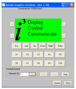
Click GO and now the user can remotely operate the  $i^3$  through the remote terminal viewer. When the user presses a button on the screen with the mouse it will operate the  $i^3$  as if the actual button had been pressed. This is a very useful tool for remote maintenance and operation.
