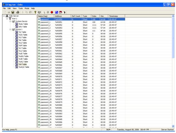
If data is being read correctly then the data items will have a green 'LED' next to them. If communications is down, then the LEDs are red. If you don't have good communications then check your cabling and the port settings detailed above. All port settings should match the settings configured for your  $i^3$ .
