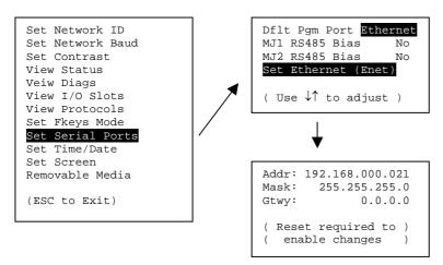
Once in the main menu, use the arrow keys to move down to Set serial ports and press enter.
