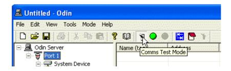
Open up the tree on the left, to reveal the data tables within each device. Click to the tables to see the data that's being read.
