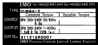
(a) Main nameplate
