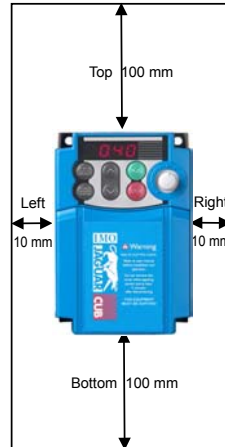
Figure 2.1 Mounting Direction and Required Clearances
