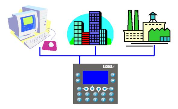
Ethernet has historically been an office "IT" network but now industrial devices have been Ethernet enabled to unite the office and factory into one standard network. This allows for a flexible, fast and global network. Also as users of office networks are able to dial into their own secured network offsite, monitoring and maintenance can be performed remotely.
