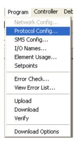
We can then configure the programmable ports of the  $i^3$ . Select either Port 1 or Port 2, however it is easier in this case to configure port 2 and leave port 1 to solely programming. Each port can have different protocols and therefore the  $i^3$  can be utilised as a data exchanger.
