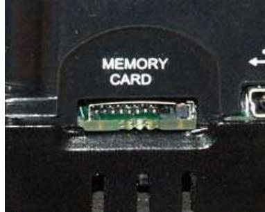
Figure 8.1 – Removable Micro SD Memory Card Slot
