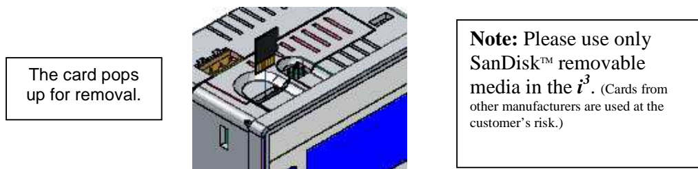
Figure 8.2 – Installing Removable Memory Card
