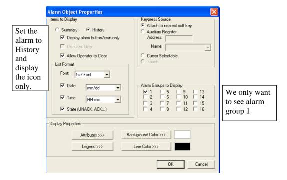
This is setting up how the alarm button will look; the actual alarm log is configured separately. When an alarm has been triggered the alarm icon will go to its ON state.
