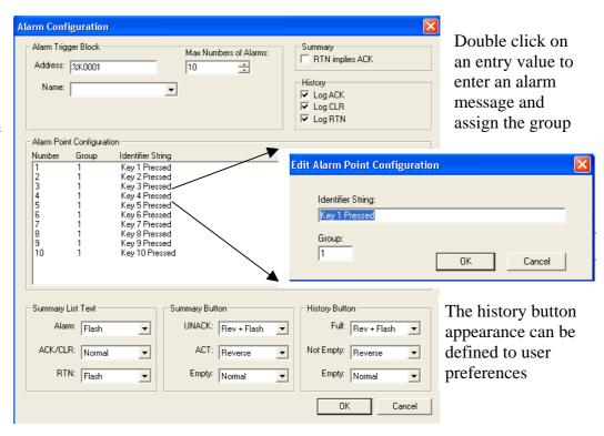
The alarms are triggered by bits, but require a 16-bit register as the trigger address. For more than one alarm group you must use consecutive registers.
