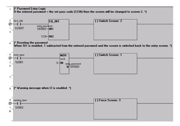
When the correct password is entered screen 2 is switched to. It will stay at screen 2, unless other logic determines, i.e. the second rung resets (switches back to screen 1). Input 2 Forces screen 3 on whilst it is enabled; when it is disabled the current screen goes back to what it was previously.
