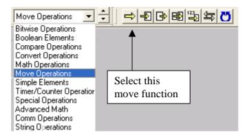
After the Move function (MOV) insert a N/O coil and assign it to the address %D01, with the Switch screen property.
